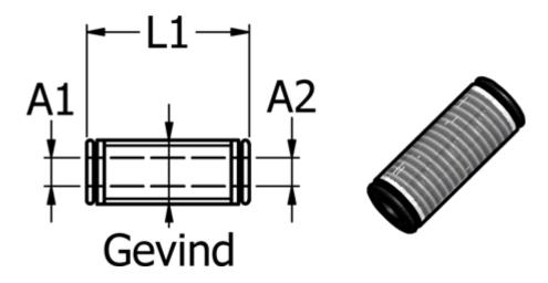
Ext. hose diameter A1 = 10 Ext. hose diameter A2 = 10 L1 = 39.2 Thread = M17x1
